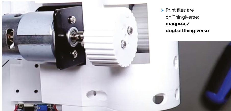
▼ The motor controller can be seen to the left, with the motors themselves in the centre of the image
