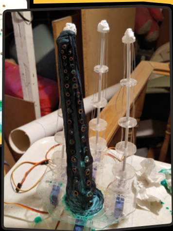
Each tentacle is controller by servos that run on a sine wave pattern to make them move more 'naturally'
