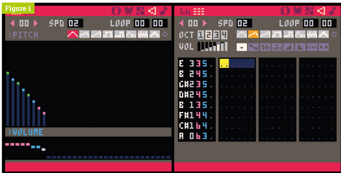
▲ Figure 1 Here's the same laser zap sound viewed in pitch mode (left) and tracker mode (right)
