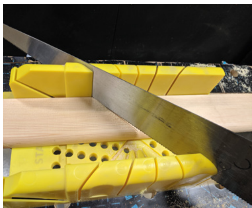
▶ Mitre boxes are very handy for cutting perfect angles on your wood
