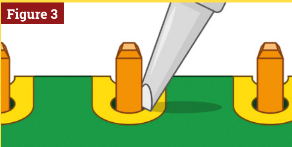
▲ Figure 3 Heat the pin and pad
