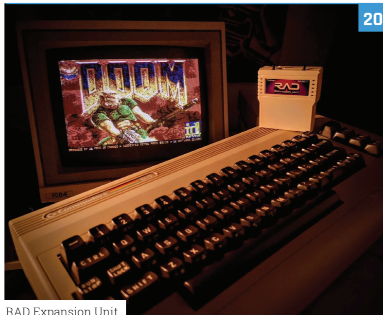
RAD Expansion Unit
