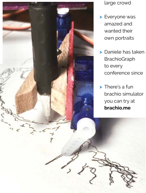
▲ The project builds on similar principles to those of a pantograph plotter
