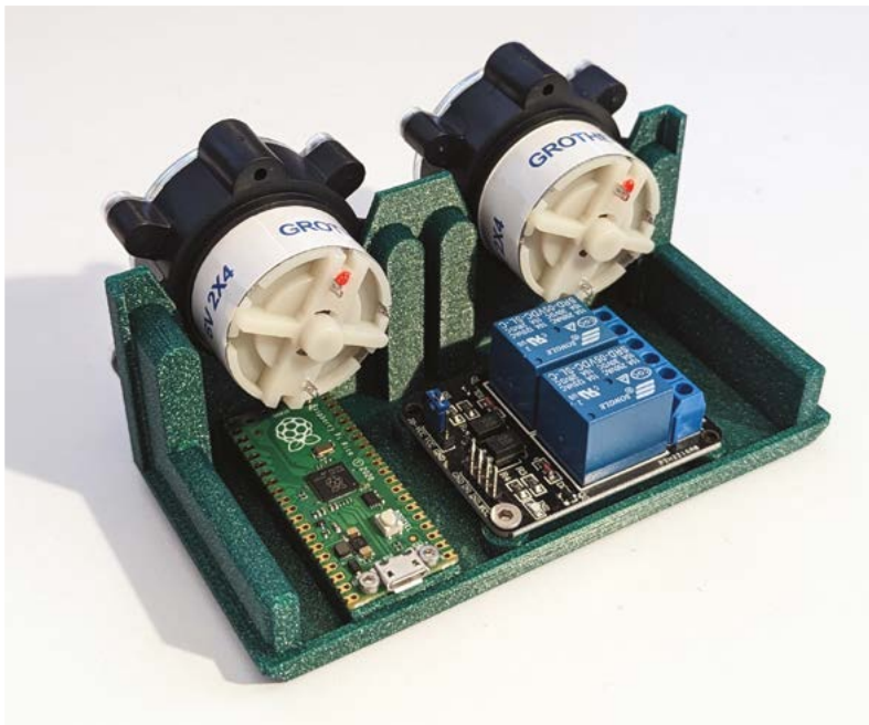
▲ The dosing heads cost just £5 each. Add Raspberry Pi Pico, a £3 relay, and £3 of wiring, tubing, soldering, plastic, and screws, and you have a very cheap dosing pump!
